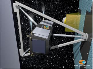
be driven through the CoG of the client satellite. The Kinitron® is sized for performing station-keeping duties for about 8-10 Months and has 60-70 kg total mass. After the 10 months it is being refueled
