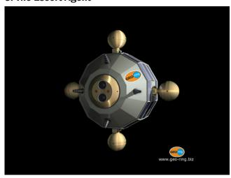
Is a miniature (7-15 kg) highly compact free-floating inspector. It is usually carried by a UA for long trips and is deployed close to the inspection target. It can perform risk free close-up inspection and relays video feed with wireless technology to the UA. Its propulsion is based on heated-gas MEMS-technology based microthrusters.
